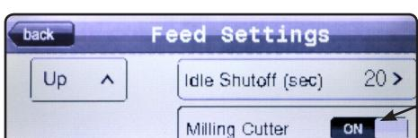
The switch indicates the current status of the milling cutter. To turn the milling cutter back on, touch the switch again until it displays “ON”.
