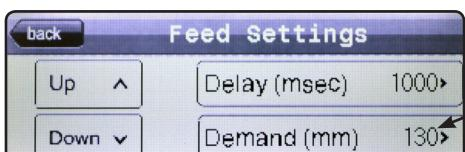
After pressing the On Demand value, a keypad will appear allowing for the number to be changed. The number must be equal to or between 30 and 400 millimeters.
